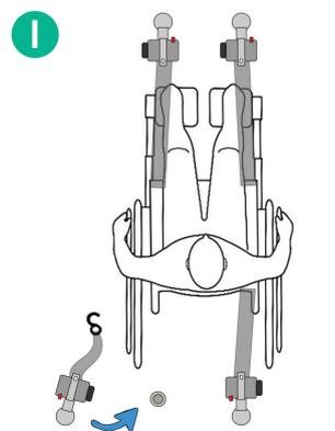
With the wheelchair in position in the vehicle, apply the brakes.
