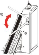
To lower the lift, insert the manual lever over the lowering valve and rotate in an anti-clockwise direction. When the platform has reached the desired position, close the valve by rotating it fully clockwise.
