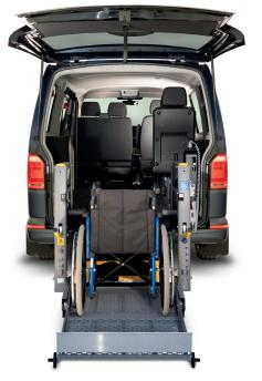
The lift is controlled by a handset on a flying lead. There are four buttons that operate different functions for the lift which are outlined below. If the remote is not illuminated, the **Up button must be pressed to wake the lift**.
